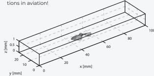
**RESULT:** 3D defect visualization after impact damage in carbon fibre reinforced plastics, for straightforward delamination detection
